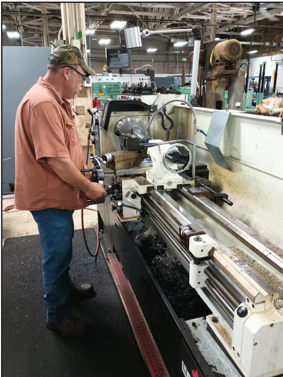
Curt Blacklock with Pine Bluff Arsenal's Directorate of Public Works, Tool and Die Fabrication area, replaces broken shafts on the pulverizer for the Thermate mixer pots on the grenade line. U.S. ARMY PHOTO BY TRACEE MILLS-DPW
