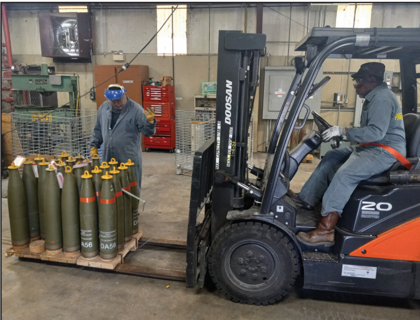
Photo above, Rex Morton (left) and Ed Moreno (right), plant operators, with Pine Bluff Arsenal's Directorate of Public Works, Waste Management and Reclamation Division, working 155mm projectile demilitarization for recycling operations.
