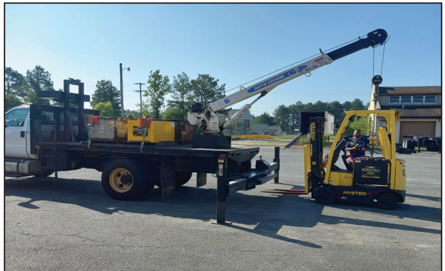
Anthony Henderson, Locomotive Engineer, with Pine Bluff Arsenal's Directorate of Public Works, Mobile Equipment Division, changes out a battery on a 4K pound electric forklift. U.S. ARMY PHOTO BY TRACEE MILLS-DPW
