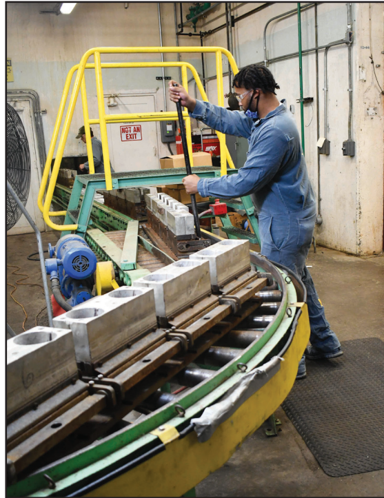
Photo left, ammunitions production worker Cadiryus White puts the AN-M14 cans in clam shell molds at the beginning of the production line. These molds fit tight around the grenade cans so it creates a funnel when the mix is added. The mix is then pressed into the cans.
