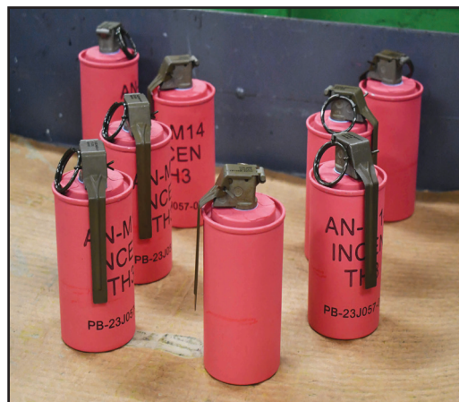
AN-M14 grenades, after they have been stenciled, stand ready to be placed in cans at the end of the production line. Thermate grenades can damage, immobilize, or destroy vehicles, weapons systems, shelters, or munitions. When the grenades are deployed, the thermate mix is converted to molten iron, burning at approximately 4,000 degrees Fahrenheit.
