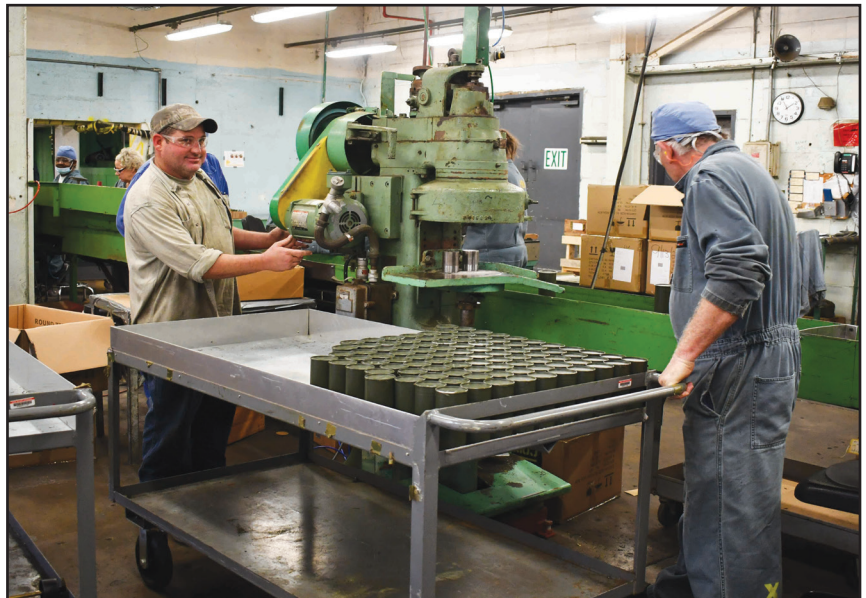
AN-M14 grenades, after they have been stenciled, stand ready to be placed in cans at the end of the production line. Thermate grenades can damage, immobilize, or destroy vehicles, weapons systems, shelters, or munitions. When the grenades are deployed, the thermate mix is converted to molten iron, burning at approximately 4,000 degrees Fahrenheit.
