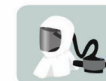
Powered Air-Purifying Respirators (PAPRs) have a battery-powered blower that pulls air through attached filters, canisters, or cartridges. They provide protection against gases, vapors, or particles, when equipped with the appropriate cartridge, canister, or filter. Loose-fitting PAPRs do not require fit testing and can be used with facial hair.
